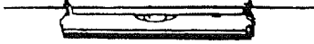
LINE LEVEL - Small tube level hangs from string line to determine level point at each corner and post.
